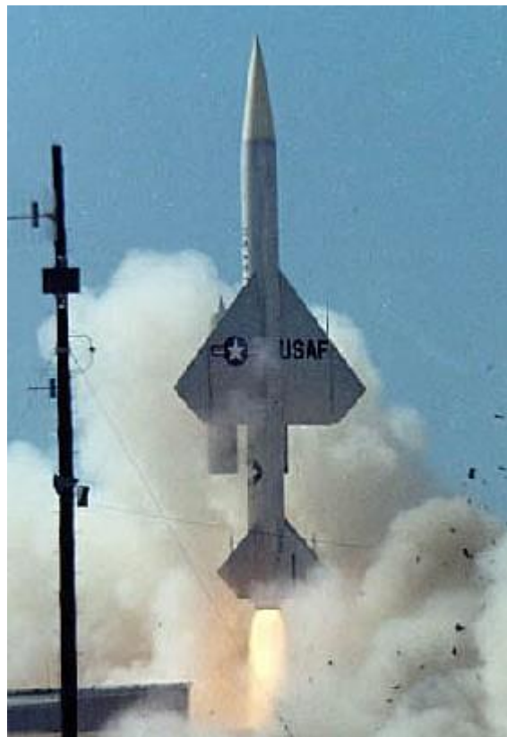
The USAF Bomarc missile cruised with ramjet engines.
