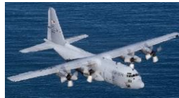
The USAF C-130 transport operates with turboprop engines.
