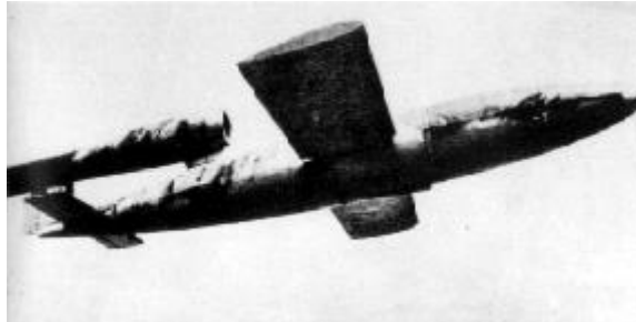
The German V-1 operated with a pulsejet engine.
