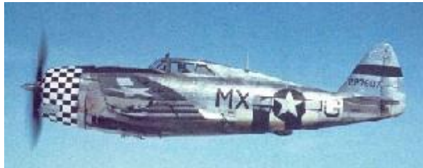
The USAAF P-47 fighter operated with a radial engine.
