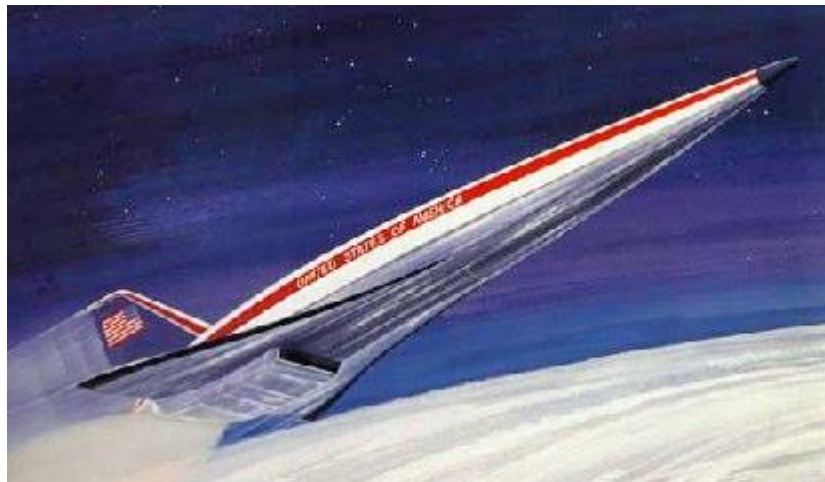
The National Aerospace Plane (NASP) will operate with scramjet engines.
