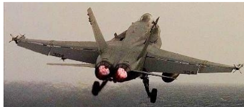
US Navy F/A-18 fighter with afterburning turbofan engines.
