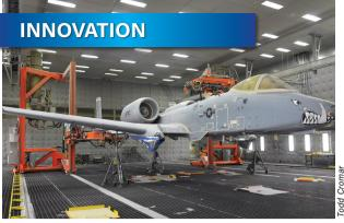
576th Aircraft Maintenance Squadron uses robotics to remove paint from A-10s to increase speed and employee safety.
