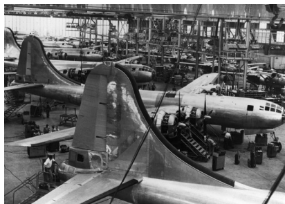
Ogden Air Materiel Area B-29 maintenance line, 1950. Some B-29s would be modified with air-to-air refueling capability.
